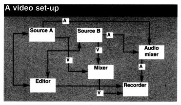
This simple djagram shows the relationship of the various items of video hardware. The 'A' signals are audio and the 'V' signals are video.
