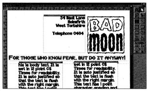
DTP programs (unlike word processors) usually work on a box system. Each graphic or block of text must have a box defined for it to exist in.
